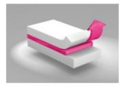
Glued joints exposed to peeling stresses are relatively at risk
