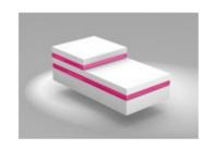
To protect the glued edges of flexible materials against peeling stress, additional reinforcing edge strips can be glued on.
