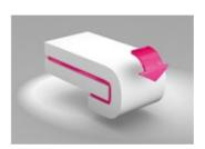
Foils glued onto rigid materials can also be protected in the edge area by taking the film down right around the edge.
