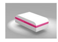
A further option for countering peeling stress is to round off the edge, thus reducing the area liable to attack.
